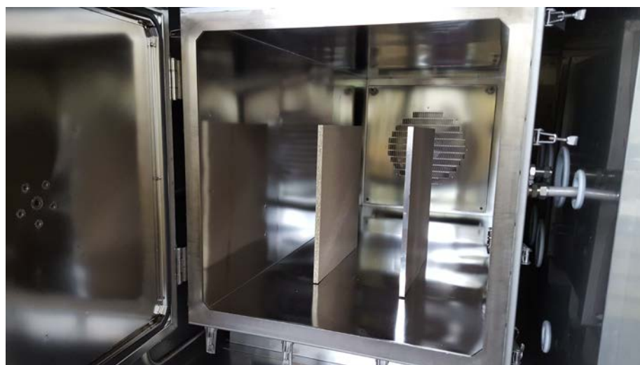
Figure 1. 1 m 3 emission test chamber with samples.
