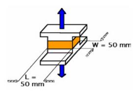
Note: Experience has shown that test specimen fixed with Hot melt often tends to affect the results. Epoxy at room temprature is considered to be the right kind of adhesive to fix the test specimen with grippers.
