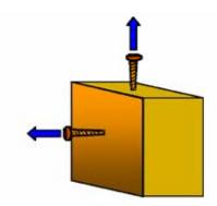
Whilst the diameter and depth of insertion of a screw will have a significant effect on the measured screw holding strength of MDF, small differences in thread form among commercially available screws would not be expected to have an effect on screw holding strength although some patented screws have advantages in production, for instance, ease of insertion.
