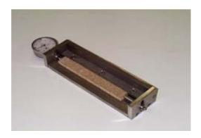
The lower limit of 35% rh, equivalent to an equilibrium moisture content of about 6% for MDF, represents the dry conditions associated with use in hot climates or in buildings with central heating. The upper limit of 85% rh, equivalent to about 13% moisture content, represents storage in a damp warehouse or the fitting out of components in a new building before the moisture has been dissipated from the building materials.
