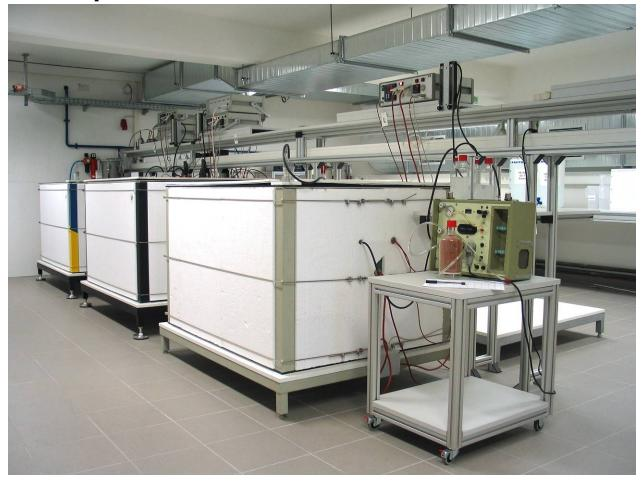
**Determination of** formaldehyde emissions ("steady state") up to 28 days in ppm or mg/m<sup>3</sup>
