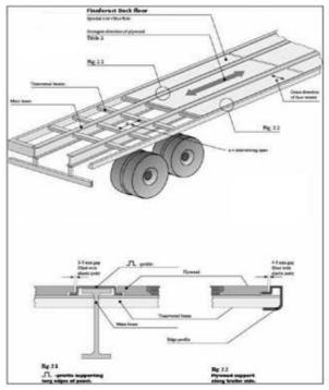
Figure 3. BirchPly Deck floor, longitudinal beams
