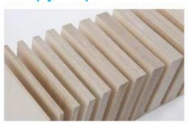
Birchply WBP Plywood is high quality light weight multi layered plywood panel made throughout from machine composed birch veneers and faced with a natural whole piece birch veneer of 1.4mm thickness. It is bonded with thermosetting, exterior quality phenolic resin adhesives commonly known as WBP (Weather and Boil Proof) and is compliant California ARB regulations on formaldehyde emissions. It also complies with European E1 standard.
