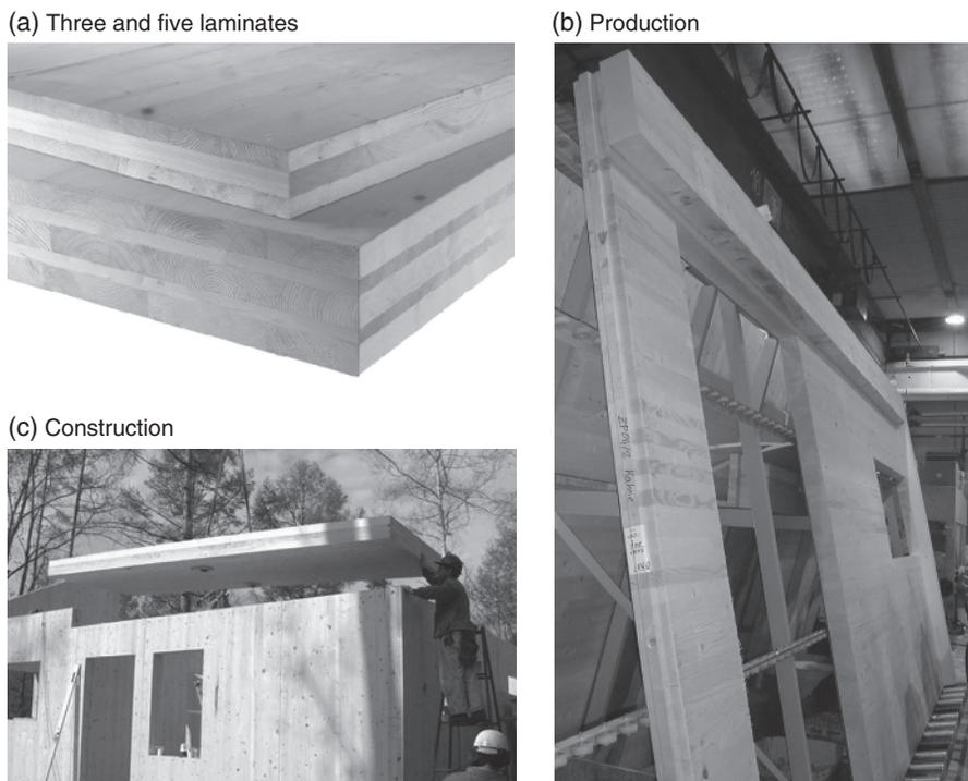
**Fig. 1.9.** Cross-laminated timber.
