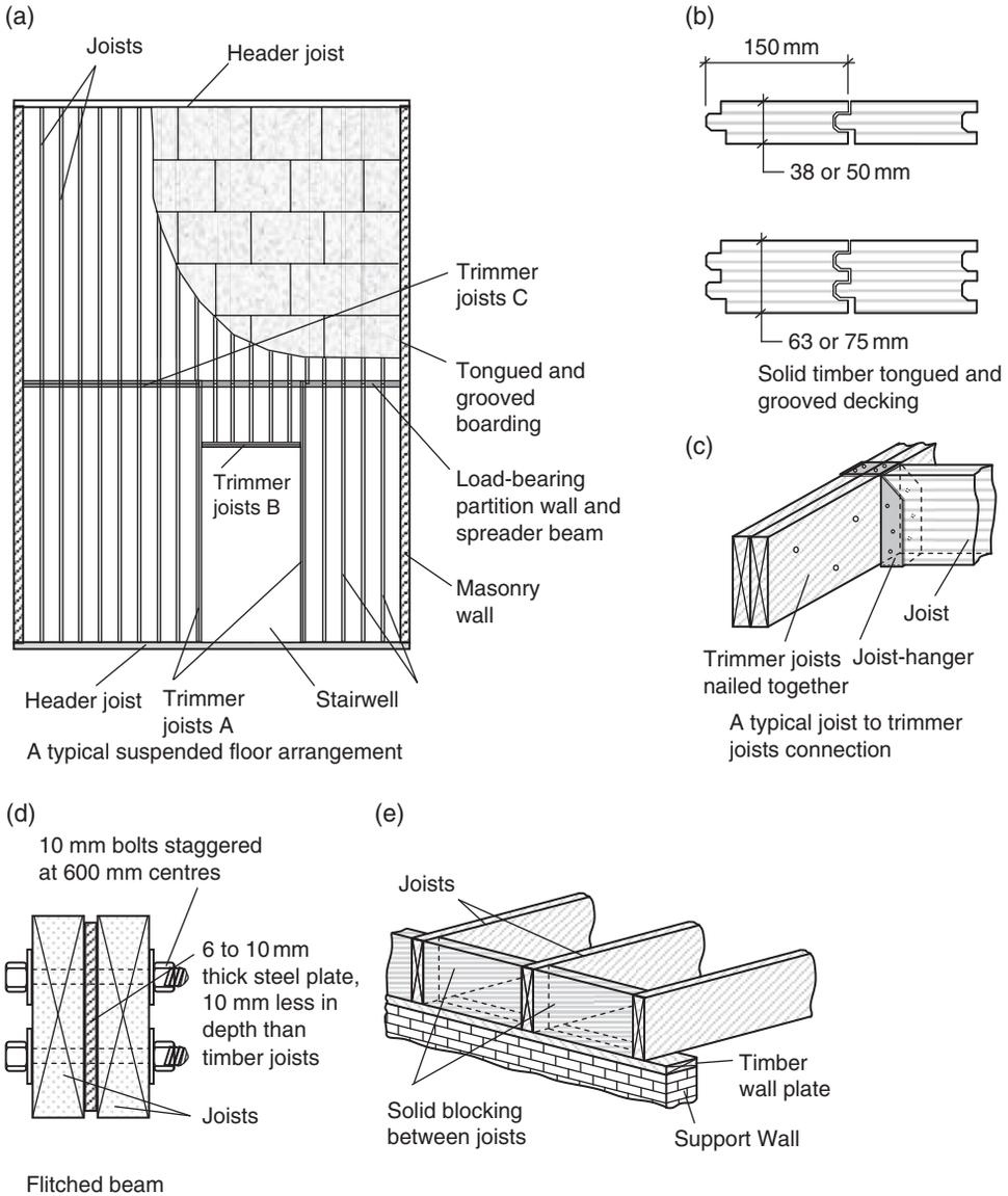
**Fig. 1.19.** Suspended timber flooring – typical components.
