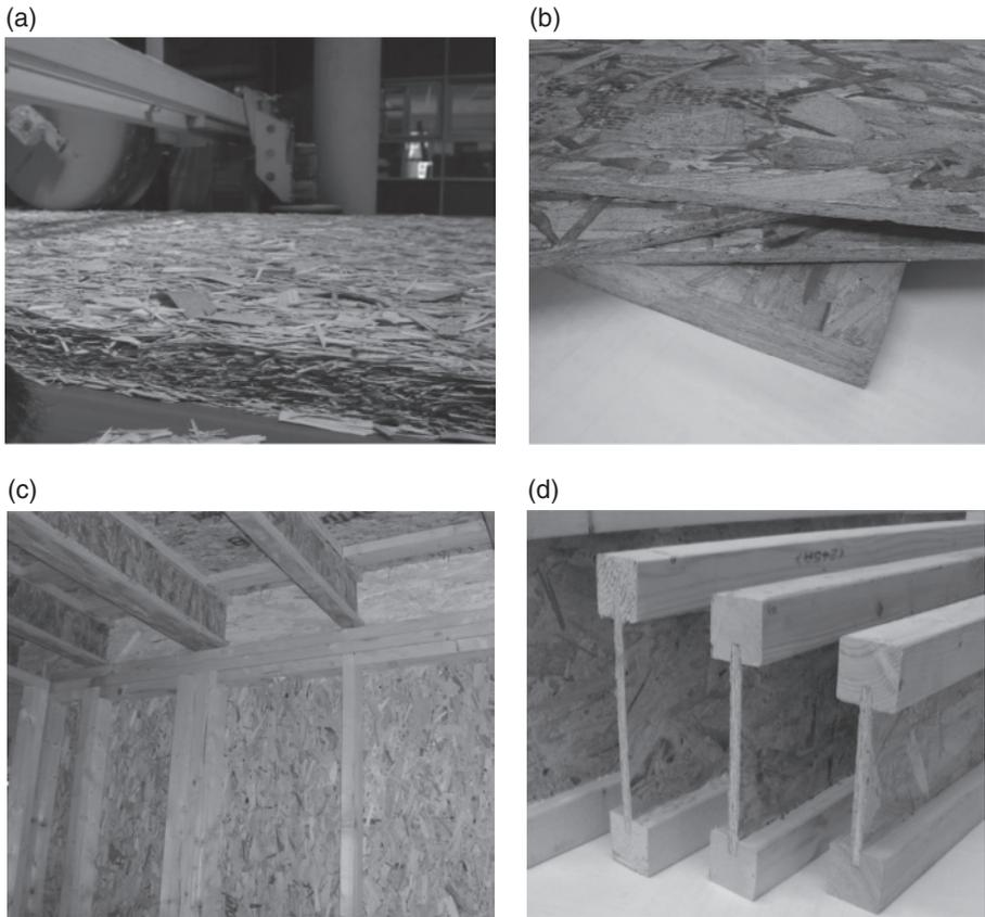
**Fig. 1.15.** OSB: (a) production before the press (photo courtesy of Wikipedia Foundation); (b) and (c) OSB boards and wall panels; (d) OSB webs in I-joists.
