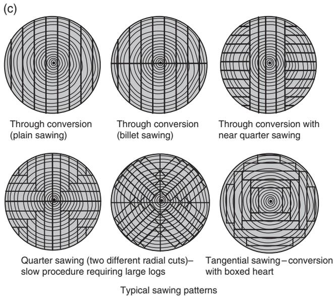
**Fig. 1.3.** Examples of log breakdown and cutting pattern.
