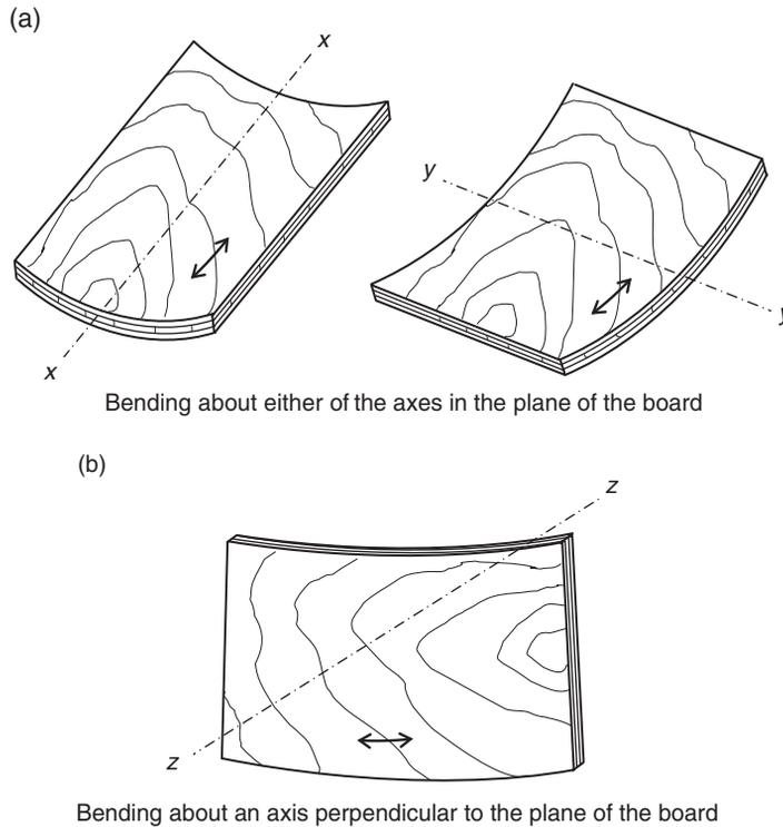
**Fig. 1.11.** Plywood – axes of bending.
