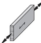
Compression or tension parallel to grain:
