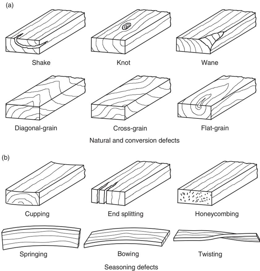
**Fig. 1.6.** Defects in timber.
