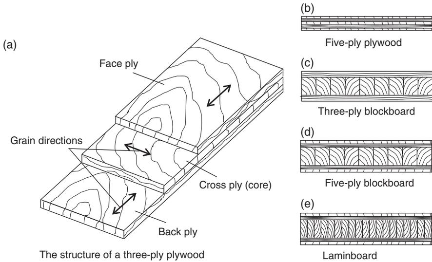
**Fig. 1.10.** Examples of plywood and wood core plywood.
