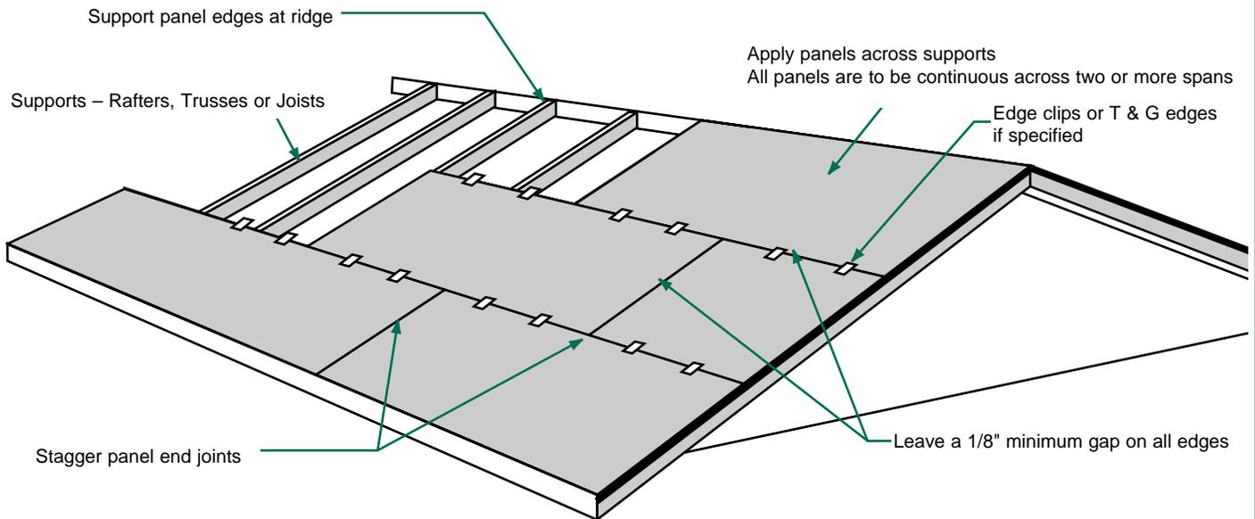
Warning: Roof sheathing may be extremely slippery when wet, covered with frost, snow, ice or sawdust. Installers of roof sheathing should wear rubber-soled footwear and exercise caution, especially on roof slopes exceeding 4 in 12. Based on recent studies, soles of thermoplastic rubber provide the best traction of the sole materials tested. Place screened surface of panel face up.
