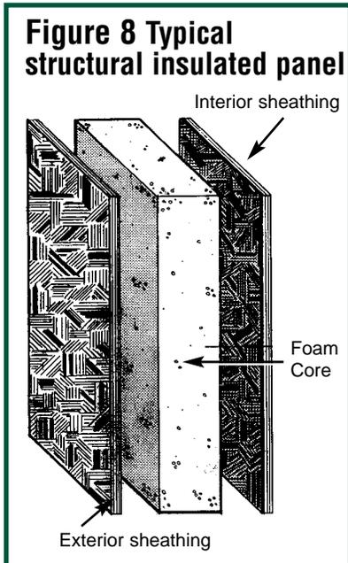
provide an alternate solution for owners and builders concerned with energy efficiency and dwindling natural resources. These panels are manufactured in sizes from 4'x 8' to 8'x 24' and have quality certified OSB faces glued to either precast or foamed in place rigid foam cores. They are manufactured throughout the U.S. and Canada in
