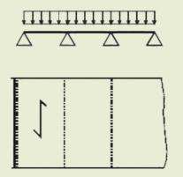
Short-term loading Service Class 3  $k_{mod} = 0.70$   $k_{def} = 0.40$   $y_q = 1.2$   $y_m = 1.3$ q given in kN/m<sup>2</sup> u given in mm
